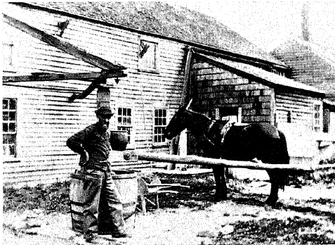
2. Pug mill turned by a horse at pottery of Asa B. Lamson, Exeter, N.H.
